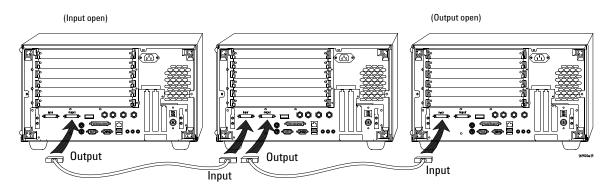
One frame's output is connected to the next frame's input. Connect multiple frames in sequence with the final frame having no output connected.
