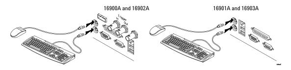
**2** Connect a monitor to the back of the 16900A. A second monitor on the 16901A, 16902A, or 16903A is optional.
