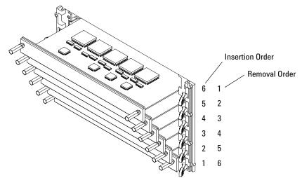
**5** Seat the modules then rotate the ejector tabs to the locked position. Repeat for all modules or filler panels.
