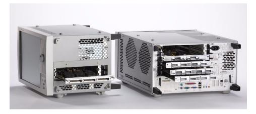
The Agilent Technologies 16900 Series logic analysis systems are modular systems with slots for logic analyzer and other types of measurement modules.
