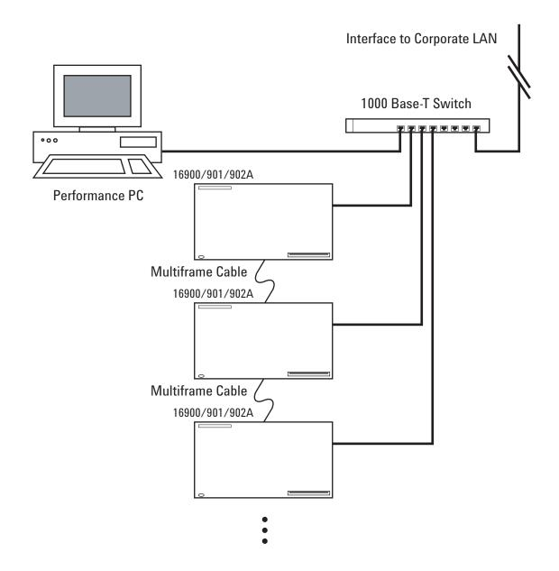
In the performance multiframe configuration, you run the *Agilent Logic Analyzer* application on a high-performance PC or server. This is useful if you trying to maximize multiframe logic analysis system performance.
