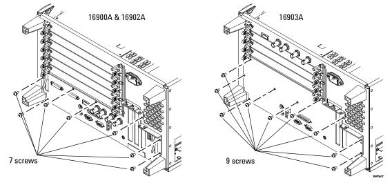
**4** Remove screws from the back of the CPU tray using a Torx T-10 screwdriver.
