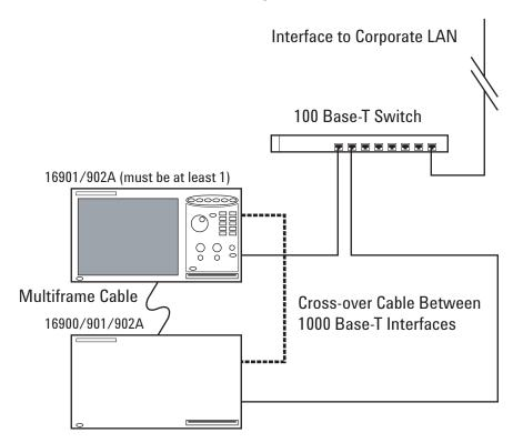
When you have only two frames in the simple 100 Base-T multiframe configuration (see page 63), you can gain performance by connecting a crossover cable between the frames' 1000 Base-T ports and configuring these ports with static IP addresses.
