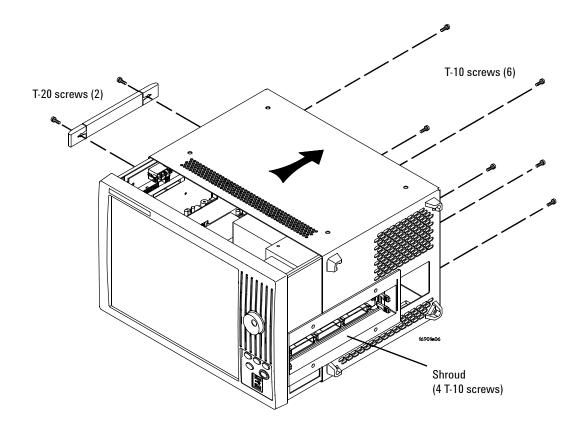
**3** For the interface card location you will be using, using a Torx T10 screwdriver, remove the screw securing the slot cover; then, remove the slot cover.
